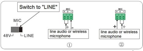
Balanced connection: "+" connects to positive, "-" connects to negative and "=""
