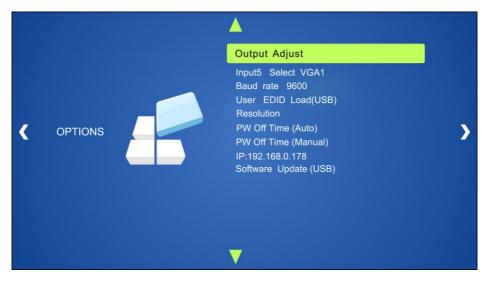
**Output Adjust**: Adjust output image position (X: horizontal direction and Y: vertical direction), ratio aspect (width and height), polarity adjustment (H Polarity and V Polarity) and output setting (HDMI on/off and HDBT on/off).
