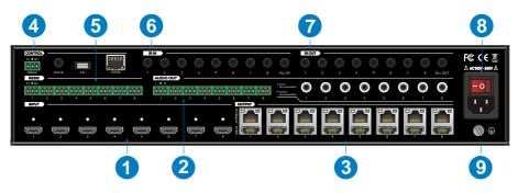
(1) INPUT: Eight Type A female HDMI input ports to connect HDMI sources.
