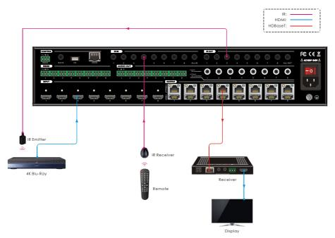
Example: Switch HDMI input 3 to HDBaseT output 2, 3, 4.
