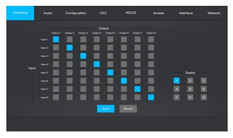
Use the 8x8 button grid on the page to set which inputs are directed to which outputs. For example, clicking the button on the Input 1 row and Output 2 column, directs input 1 to output 2.
